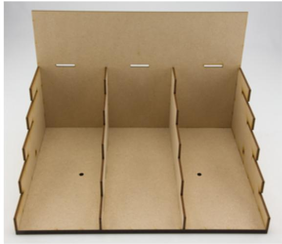
6. Glue the shelves into place. Note that the top shelf has tongues that fit into the rear. Also the depth of the cut out increases towards the top, i.e. the second shelf has a greater cut out than the third shelf..
