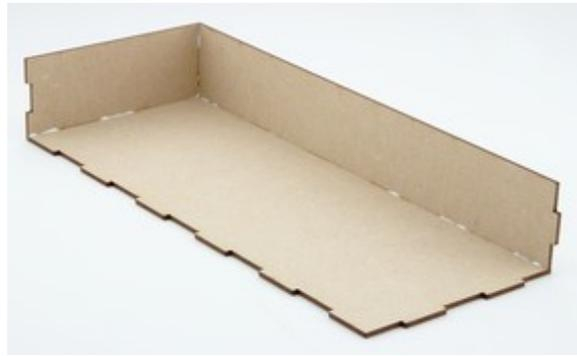
3. Glue the second side on. Remove any excess glue to ensure that the drawer will run smoothly.
