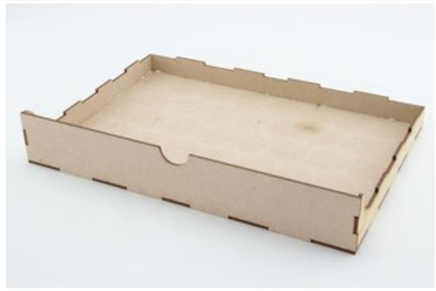
4. Glue one spacer to the rear of the front, below the cut-out. This will support the top.
