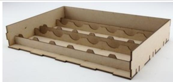
4. Glue the front on. Make sure that this is glued on well as you'll be pulling the weight of all the paints with this.
