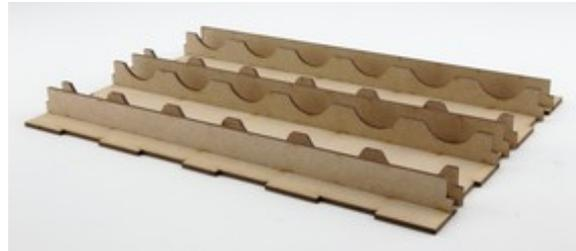
2. Glue the two sides on. Don't forget to dry run, it makes it much easier. Also remember to remove excess glue to ensure smooth running of the drawers.
