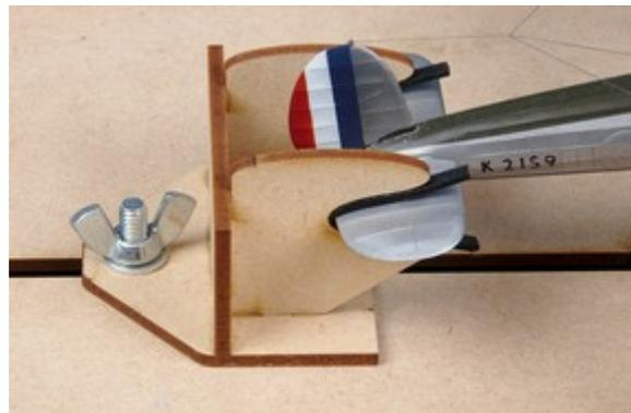
3. The upper wing supports locate into the remaining long slot. Set one of the supports to hold the wing in the required location and then use the graduation markings to set the second support up to match it. It is probably worth using white tack to gently attach the upper wing to the supports.
