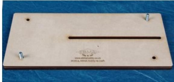
2. The extension is attached to the main base by four nuts and bolts and the two smaller pieces of mdf. The extension may be attached either way around depending on the length of the fuselage.
