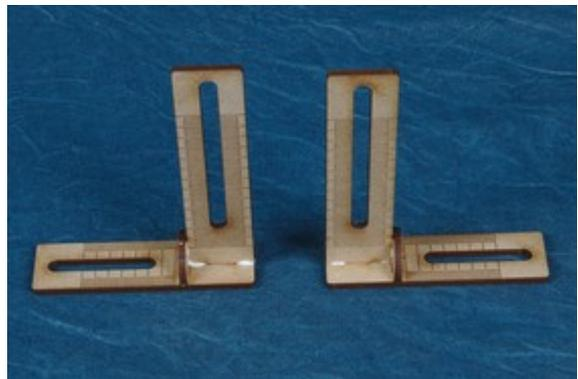
3. The L shaped wing supports bolt onto the uprights with the supports against the graduated face.
