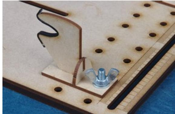
2. The tail plane clamp locates into the long slot at the opposite end of the jig. With the model located against the main plane clamps slide the tail plane clamp up to the tail plane so that the aircraft is held in position. The clamps do not have to be pushed together hard.
