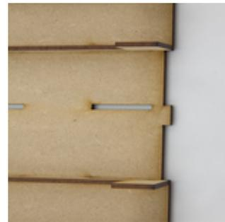
2. Position the 3mm magnets into the side panels and the 6mm magnets into the top and base. Remember the polarity of the magnets.
