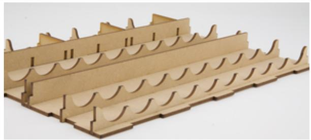
4. Glue the two sides on. Don't forget to dry run, it makes it much easier. Also remember to remove excess glue to ensure smooth running of the drawers.
