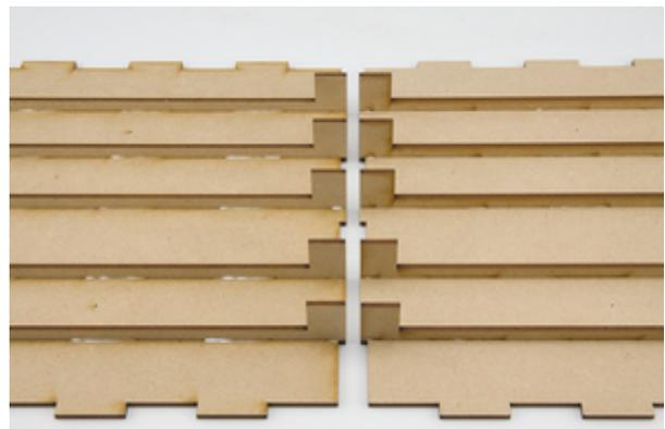
4. Glue the rear onto the base. Ensure you get it the right way up. The middle shelf slots should be to the top of the adjacent side slots.
