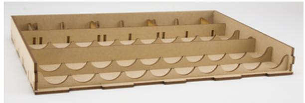
6. Glue the front on. Make sure that this is glued on well as you'll be pulling the weight of all the paints with this.
