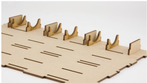
2. Place the intermediate strip with the cutouts onto the base. This does not need to be glued.
